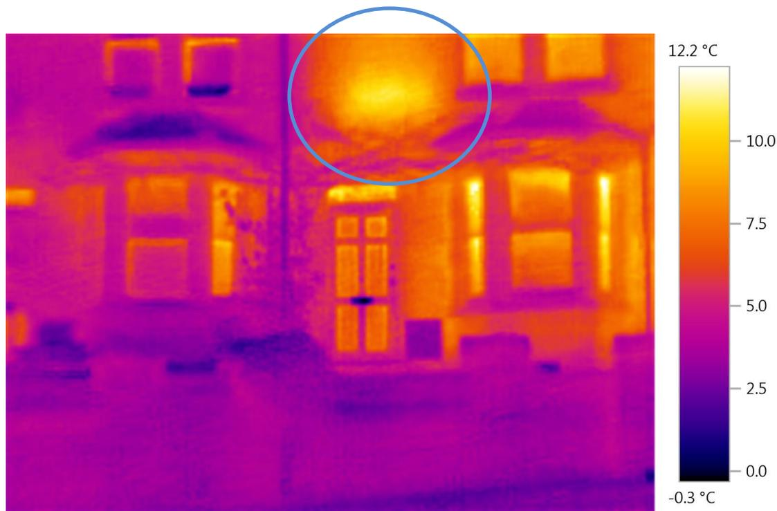
This is a common sight in Bath with radiators on outside walls of solid walled homes. It will also affect homes with uninsulated cavities, but this will be less obvious with the camera as the heat will be dispersed within the cavity. The owner should fit (Radflek) radiator reflectors.
