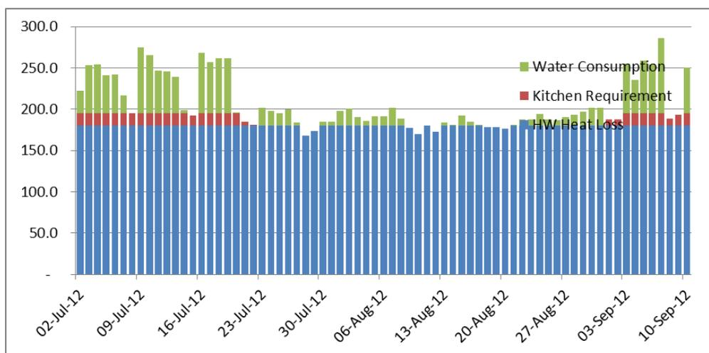
either side of a summer holiday when the school was unoccupied. The green represents hot water consumed by the school, the blue the gas consumed just to keep the system running – losses from the circulatory hot water system. The system is less than 20% efficient – it should be at least 90% efficient.
